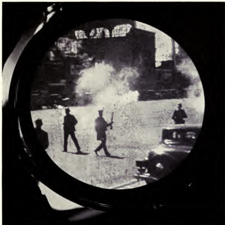
Fig. 73. A Scene Projected in Infra-red on the Fluorescent Screen of the Image Tube
